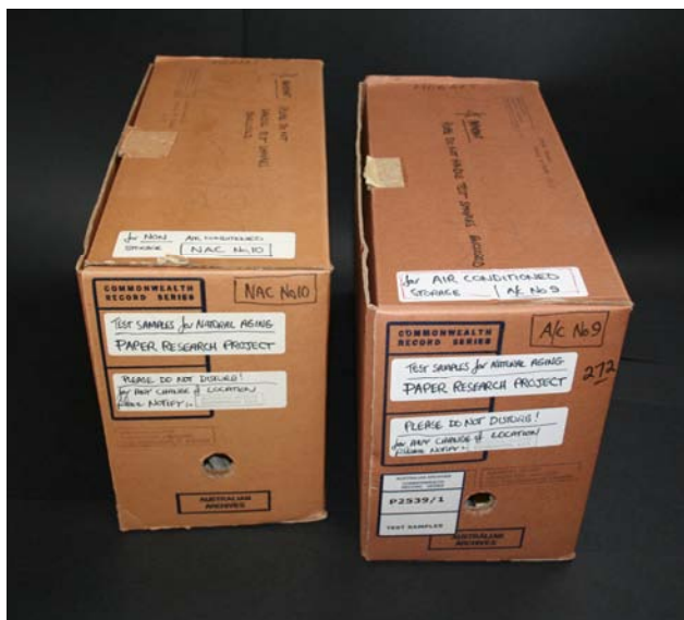
Figure 1: Comparison of box stored 27 years in non-A/C environment (left) and box stored in A/C environment (right)
