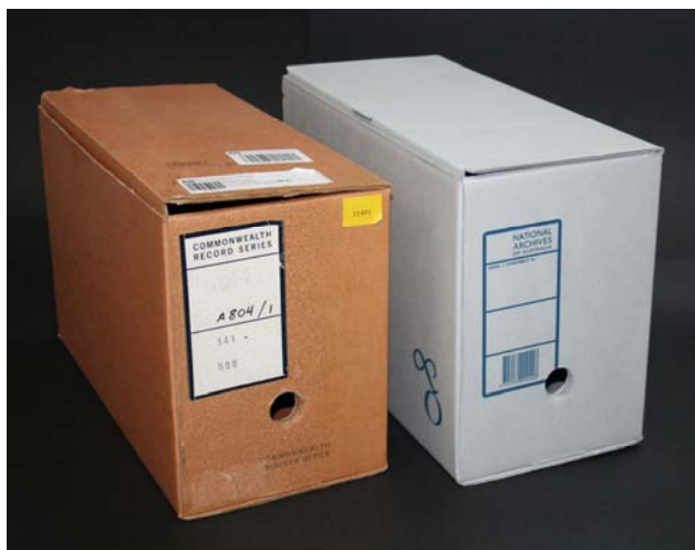
Figure 1: Type 1 boxes made from acidic brown paperboard in the 1960s (left) and buffered archival paperboard currently used (right) at the NAA
