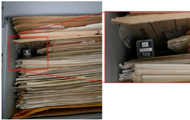
Figure 3: Internal probe in air space in a filled box
