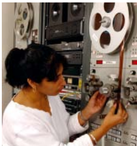
Geeta Jatania prepares to copy a magnetic soundtrack to a more stable polyester film.
