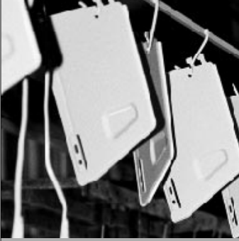
An electrostatically applied powder coating system was used at each of the plants producing shelving products for Archives II.
